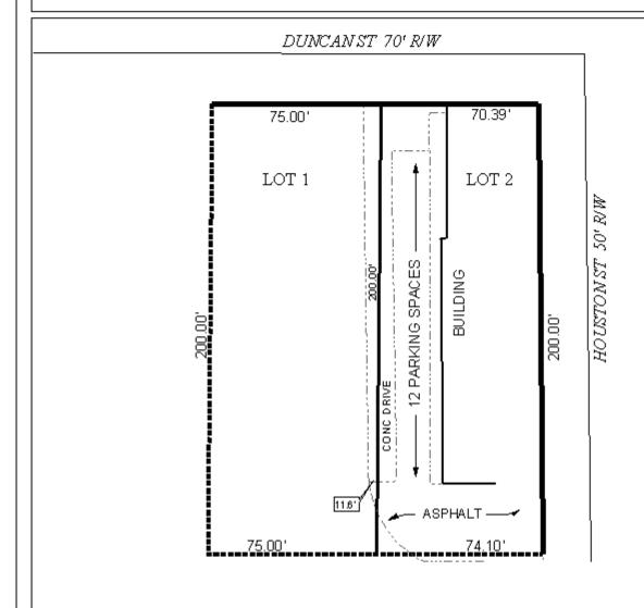
The site plan illustrates the existing building, asphalt, drive, and lot dimensions.
