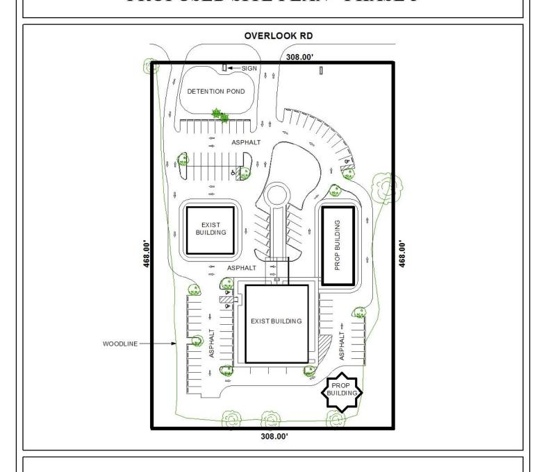
The site plan illustrates the existing buildings, proposed buildings, and asphalt drives and parking.
