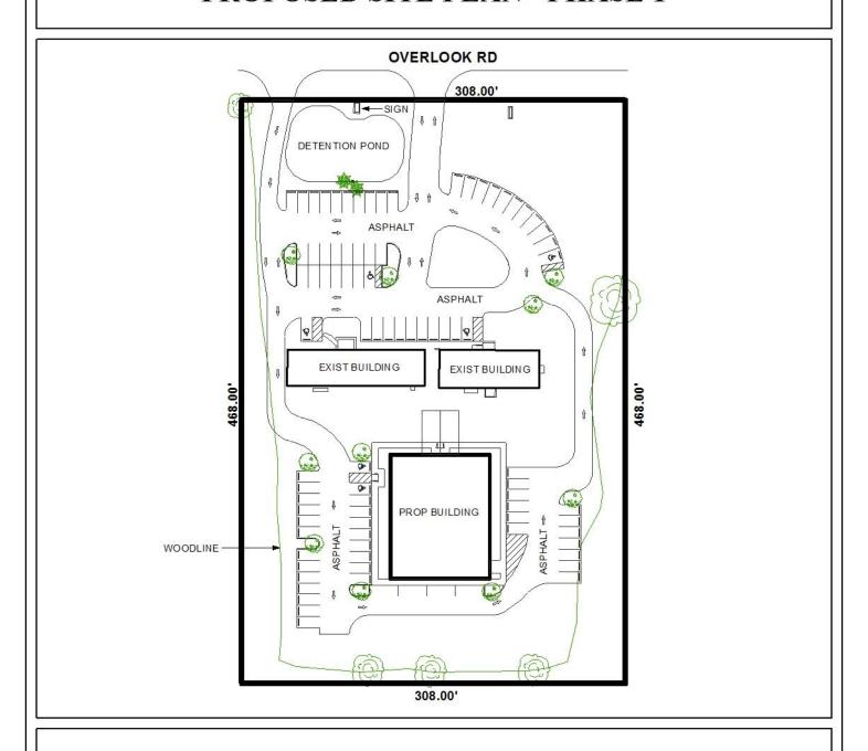
The site plan illustrates the existing buildings, proposed building, and proposed asphalt drives and parking.
