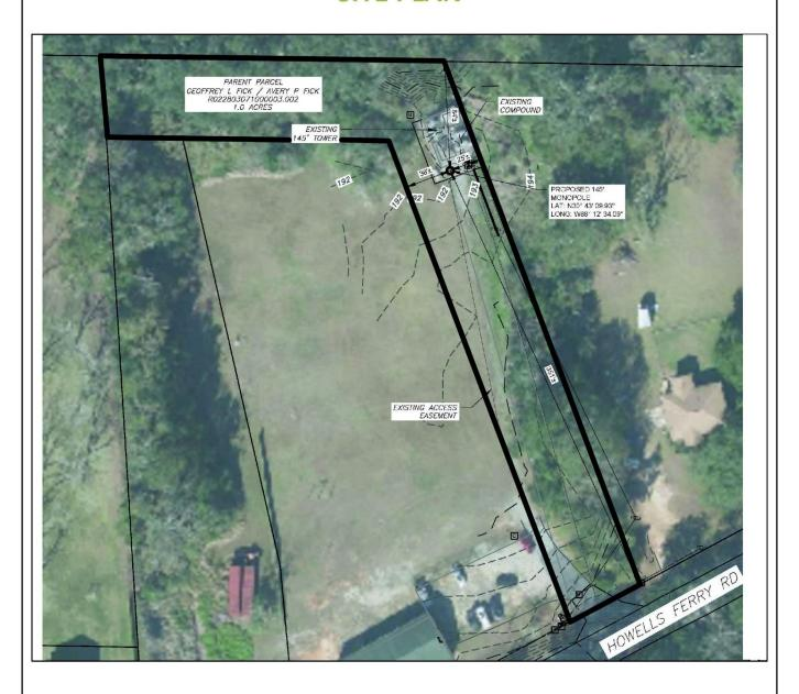
The site plan illustrates the existing tower, proposed tower, and easements.
