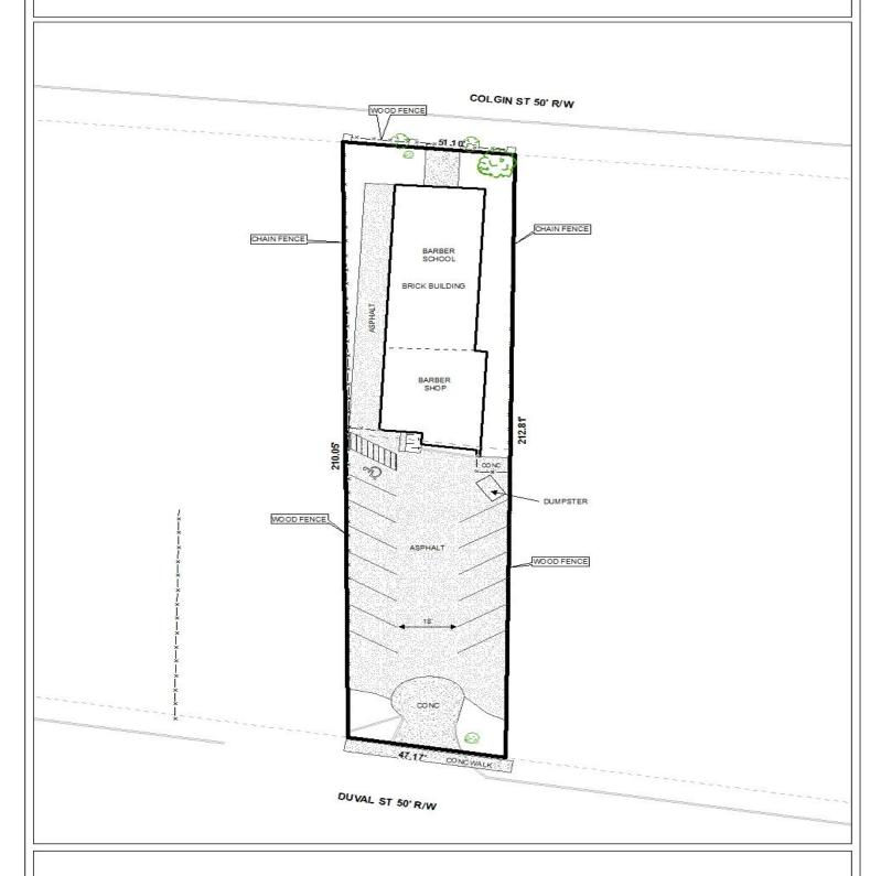
The site plan illustrates the existing building, dumpster, parking, and fences.
